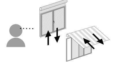
Within 5 seconds press the corresponding button (i.e. UP if the motor rotates upwards or DOWN if vice versa) on the **new transmitter being added**.
