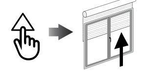
Press the STOP button to set the limit. The motor makes a brief jog to confirm. The new up limit is set.
