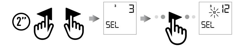
When all the desired channels of the group are set press the UP, STOP or DOWN button to confirm the group. The group is identified by a number. The group you set takes the first number available in progressive fashion from 1 to 8.
