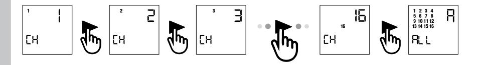
**Group control mode\***: the first group to appear is the all channels group. Scroll through the pre-made groups with the arrow buttons ( $\blacktriangleleft$  /  $\blacktriangleright$ ). Each group is identified by a number.
