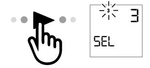
Press for 2 seconds both arrow buttons ( $\triangleleft + \triangleright$ ) to select the channel. Repeat point 3 and 4 to add other channels in the same fashion.
