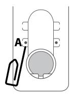
Check the rotation of the motor, then release PROG-TX (the motor stops).
