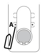
Check the rotation of the motor, then release the PROG-TX button (the motor stops).
