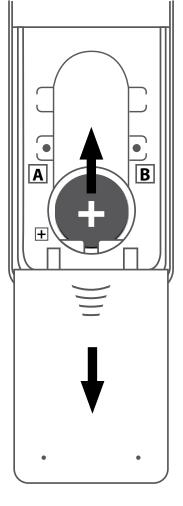
Press and hold the circle button while reinserting the battery. Once the screen comes back on and displays -ESEL, the circle button can be released.
