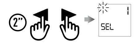
Using the arrow buttons ( $\blacktriangleleft$  /  $\blacktriangleright$ ), 3 scroll to the channel to be set into the group
