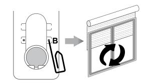
Press and hold the UP button and run the motor to the desired UP limit position.
