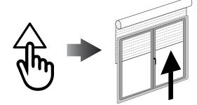
Press STOP to set the UP limit position. The motor makes a brief jog.
