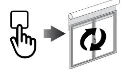
Press and hold the DOWN button and run the motor to the desired DOWN limit position.
