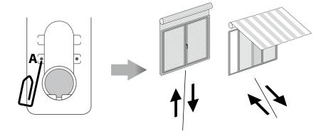
Press STOP: The motor makes a brief jog. Direction of the motor has been reversed.
