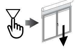
Press STOP to set the DOWN limit position. The motor makes a brief jog.
