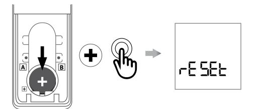
After about 3 seconds the transmitter will start up and all channels will be unhidden, and any groups deleted.
