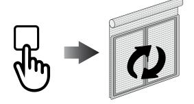
Note: accurate limit setting can be performed when UPWARD or DOWNWARD by pressing the PROG-FC button a second time. The motor then moves slowly in steps towards the desired limit. Always press STOP button to set the limit position.
