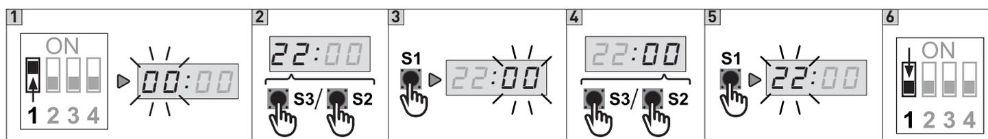
1. Put DIP 1 (S4) in ON position, PARAMETER digits start blinking
