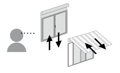
Within 5 seconds press the corresponding button (i.e. UP if the motor rotates upwards or DOWN if vice versa). The transmitter has been programmed and the rotation of the motor has been synchronized.
