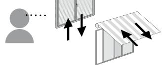
Within 5 seconds press the corresponding button (i.e. UP if the motor rotates upwards or DOWN if vice versa). The transmitter has been programmed and the rotation of the motor has been synchronized.
