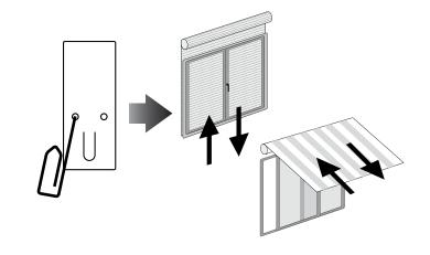
Press STOP: The motor makes a brief jog. Direction of the motor has been reversed.
