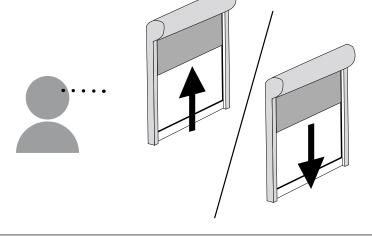
Within 5 seconds press the corresponding button (i.e. UP if the motor rotates upwards or DOWN if vice versa) on the **new tran**smitter being added.
