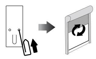
Press and hold the UP button for more than 2 seconds then release.
