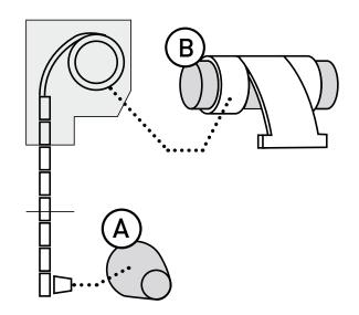
Press and hold the UP button for more than 2 seconds then release. The motor runs upward to the TOP limit, stops itself (because the bottom bar beats against the cassette) and sets the TOP limit.
