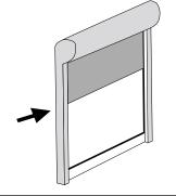
Press simultaneously the UP and DOWN buttons until the motor makes a brief movement in both directions.
