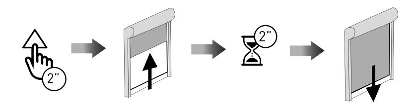
To double check make a full TOP/BOTTOM cycle of the roller shutter
