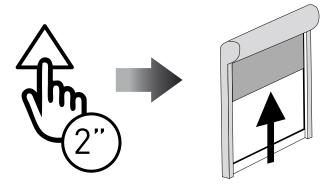
When you reach the TOP limit position press STOP. The motor stops.
