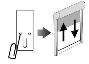
Press STOP: The motor makes a brief jog. Direction of the motor has been reversed.
