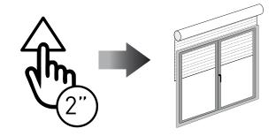
When you reach the TOP limit position press STOP. The motor stops.
