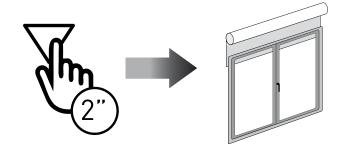
When you reach the DOWN limit position press STOP. The motor stops.
