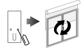
Press and hold the UP button for more than 2 seconds then release. The motor runs upward to the TOP limit, stops itself (because the bottom bar beats against the cassette) and sets the TOP limit.
