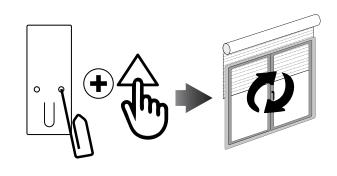
Press and hold the UP botton until the desired new UP limit is reached.
