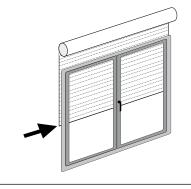
Press simultaneously the UP and DOWN buttons until the motor makes a brief movement in both directions. The intermediate position has been setup.
