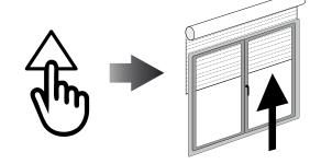
Press the STOP button to set the limit. The motor makes a brief jog to confirm. The new up limit is set.
