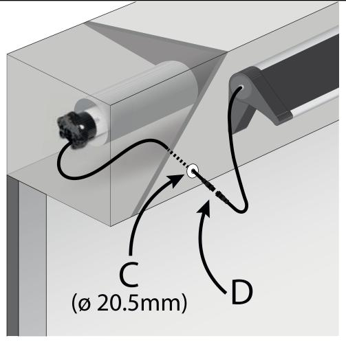
The motor cable is equipped with a cable gland (C) which can be mounted on sheet metal with a thickness of 0.5 to 3 mm by drilling a hole ø 20.5 mm.
