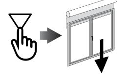
Press the STOP button to set the limit. The motor makes a brief jog to confirm. The new up limit is set.
