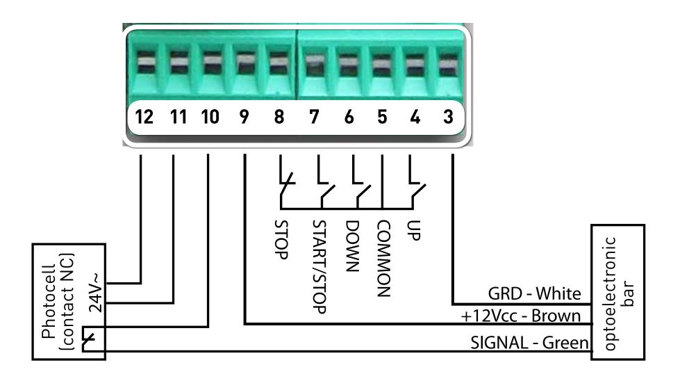
To connect the the photocell, the latter must be connected as shown (**DIP 4 in OFF**).
