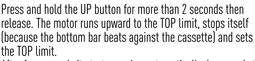
After few seconds it starts running automatically downwards to self-set the BOTTOM limit.
