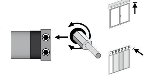
In case you need to correct the "up" limit position, because it's over, close the shutter/roll the awning down) shortly, then turn the upper adjusting screw to . Repeat then the sequences from point 3.
