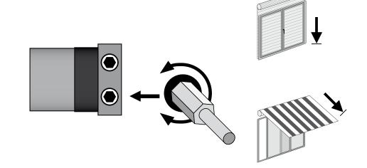
Open the shutter/roll up the awning until it does not stop and then turn the upper screw to till the shutter/awning reaches the exact desired "up" position.
