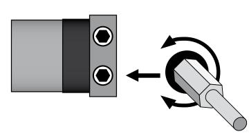
Fixing the shutter/awning at the tube and then turn the lower adjusting screw to • or • in order to set the exact desired "down" position.
