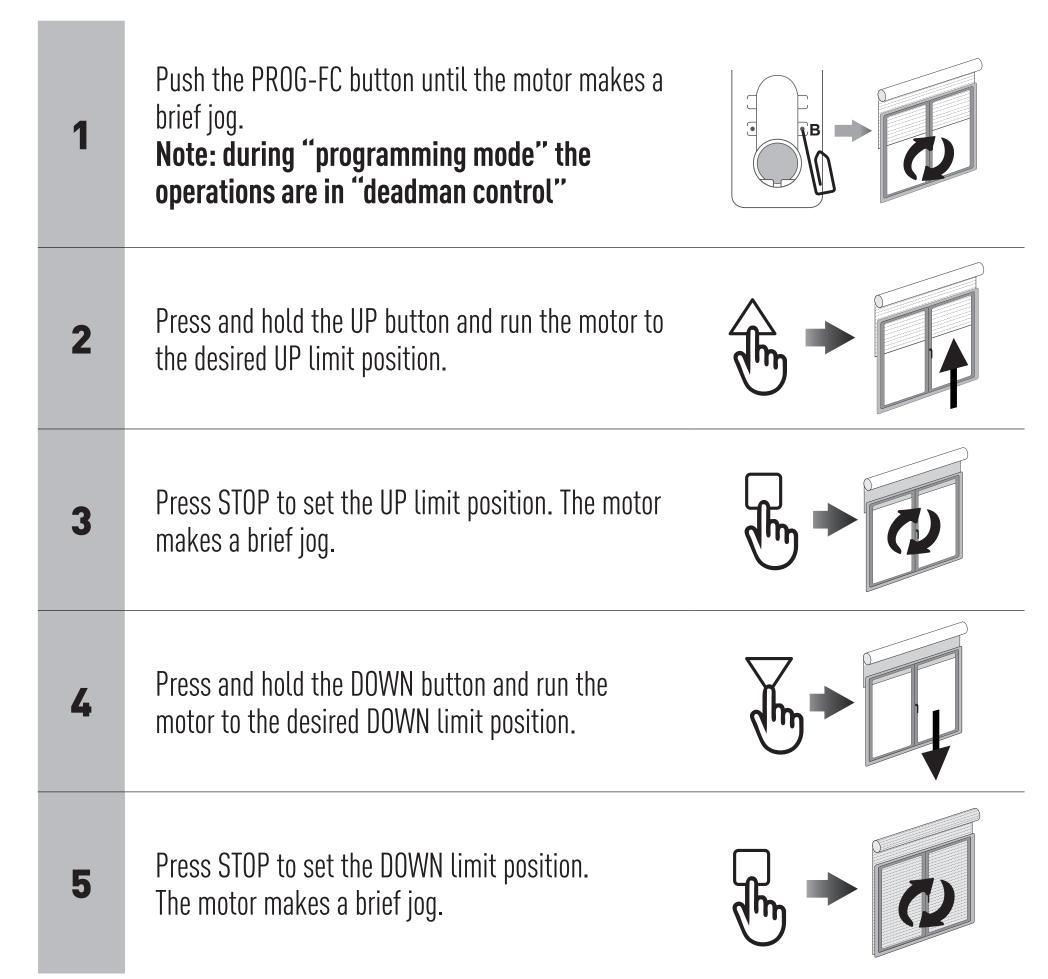
Note: accurate limit setting can be performed when UPWARD or DOWNWARD by pressing the PROG-FC button a second time. The motor then moves slowly in steps towards the desired limit. Always press STOP button to set the limit position.
